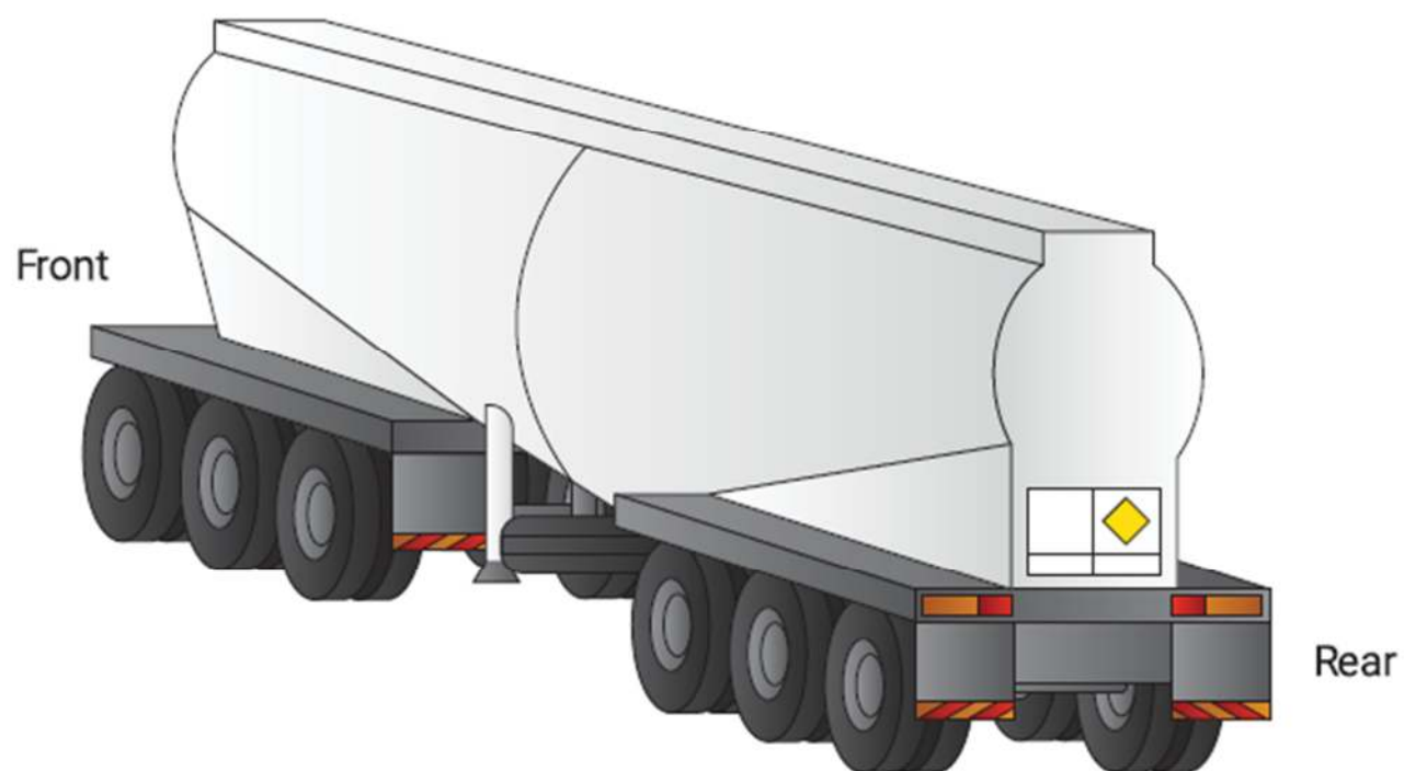
Figure 4.5 Representation of the tanker trailer, demonstrating the four tyres on each axle (12 at the rear and 12 under the dolly at the front)
