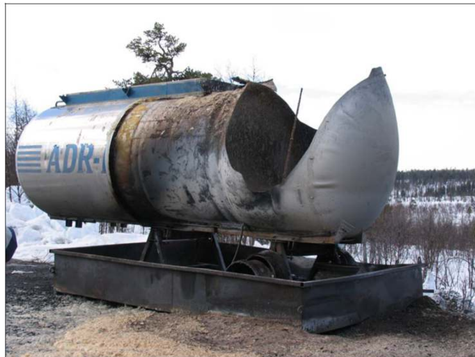
Figure 15, shows the ruptured stainless steel tank after the fire test. The rod is connected to the bottom valve and is a part of the tank.
