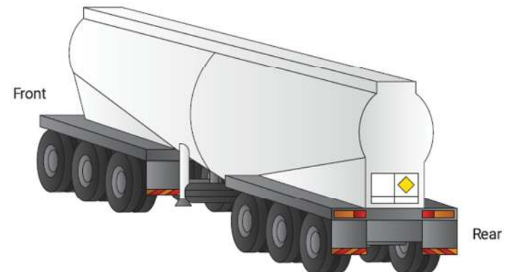
Figure 4.5 Representation of the tanker trailer, demonstrating the four tyres on each axle (12 at the rear and 12 under the dolly at the front)
