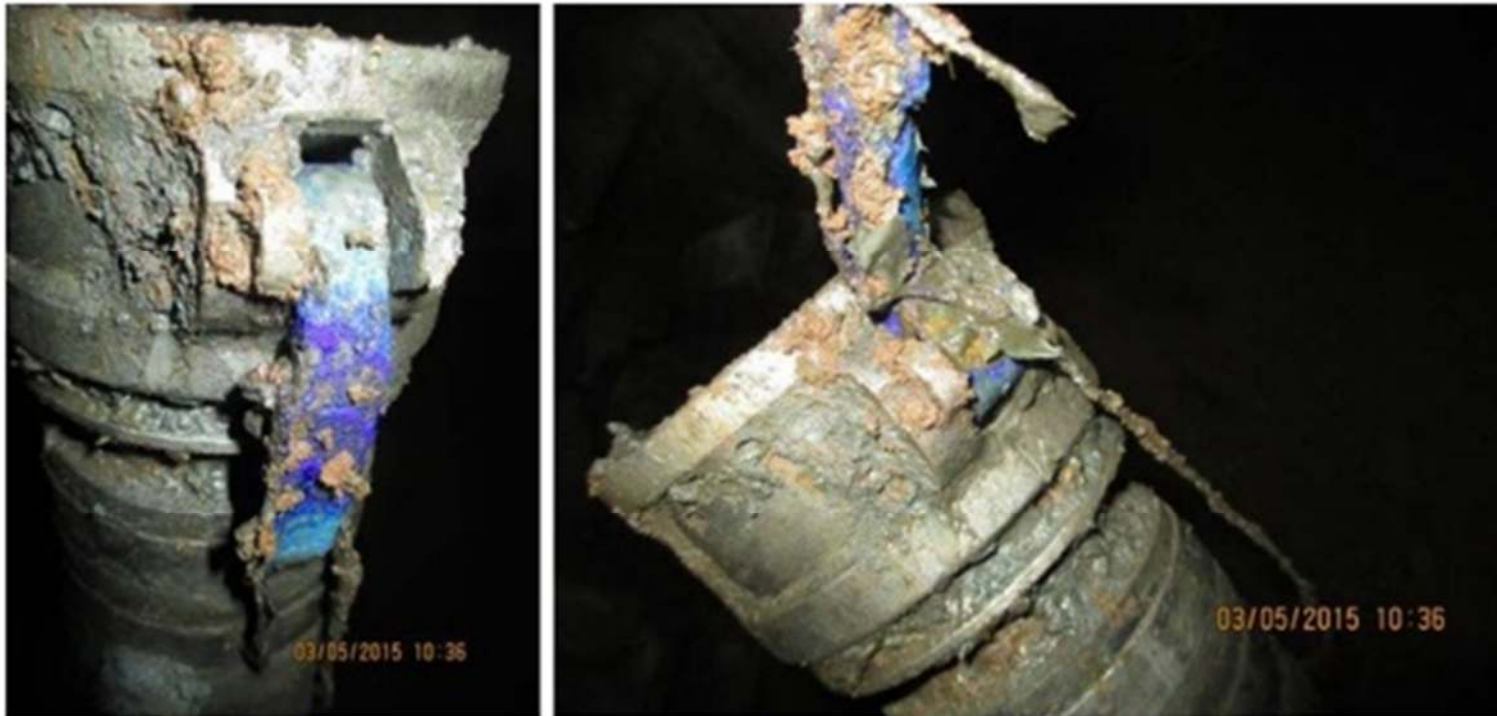
Image 1 - TACN on brass locking lever of cam-lock
