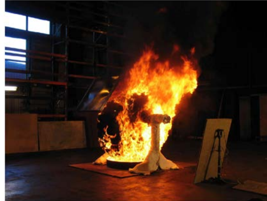
Figure 9 A photo taken after 4:16 minutes from ignition. The heat release rate is about 2 MW. The peak heat release rate was 2.3 MW, reached at 3 minutes after ignition.
